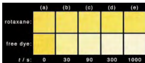
Figure 4. Photographs of cotton samples dyed with rotaxane 1 (top) and free dye 3 (bottom), before (a) and after different times t of bleaching with \text{Na}_2\text{S}_2\text{O}_4 (1M): b) t = 30 , c) t = 90 , d) t = 300 , e) t = 1000 s.
