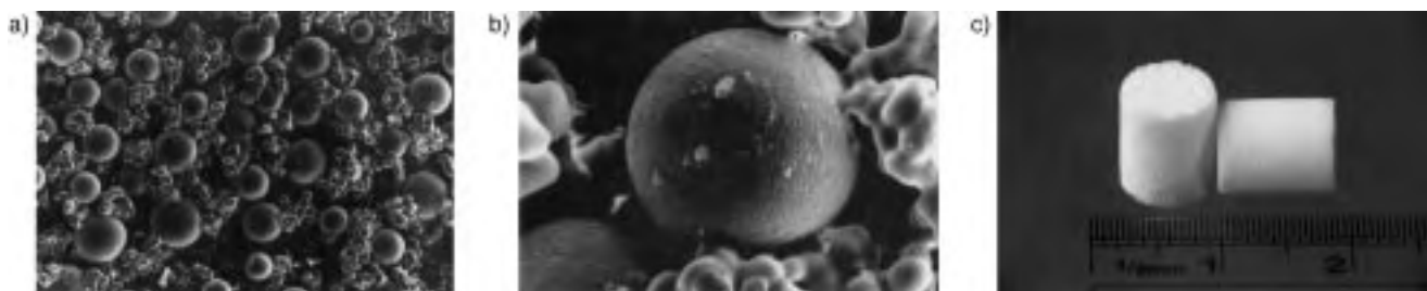
Figure 1. a) Cross-section of resin plug (100 \times magnification). b) Single bead within the matrix of resin plug (270 \times magnification). c) Illustration of dimensions of resin plug (9 mm long, 7.5 mm diameter).
